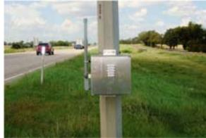
Post Oak Traffic Systems revolutionary traffic detection device reads MAC addresses from enabled Bluetooth devices and forwards them to software capable of estimating travel times and speeds.
